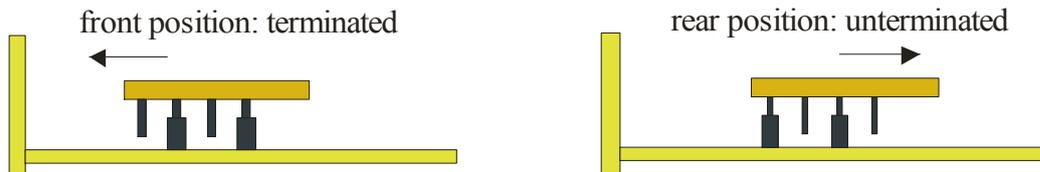
The differential jumper set allows for differential input signals (ECL, LVPECL, LVDS). The unipolar jumper set allows for unipolar signals (NIM, TTL, analogue positive or negative signals). A threshold of  $\square 1.5\text{ V}$  can be set in 256 steps. The polarity is chosen to allow NIM triggering at the leading edge with "positive edge" setting (default). For TTL signals "neg edge" should be selected.
