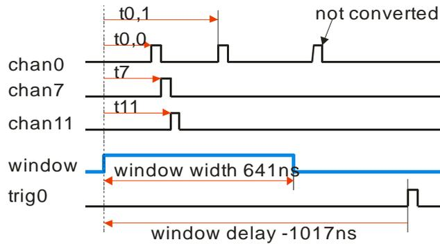
The trig0 -1017 ns is the virtual start for the data. Channel resolution is selected to 1/64 ns (15.6 ps)
