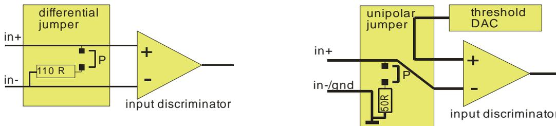
"P" means jumper position near to front panel, then input is terminated.
