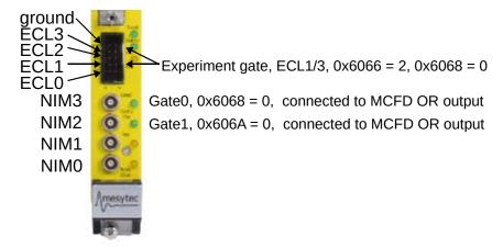
Set NIM3 = gate0, NIM2 = gate1 0x6068 = 0 //Gate\_select  $\rightarrow$  Gate 0 and 1 from NIM-inputs 0x606A = 0 // NIM\_gat1\_osc, Lemo2 is  $\rightarrow$  gate1 input
