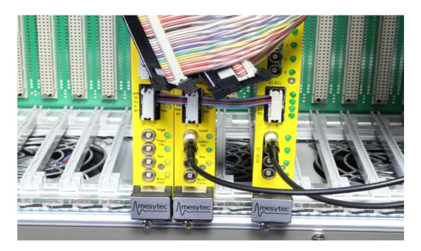
The picture shows the ECL bus which provides the experiment gate to MQDC and MTDC. it is terminated at the end.
