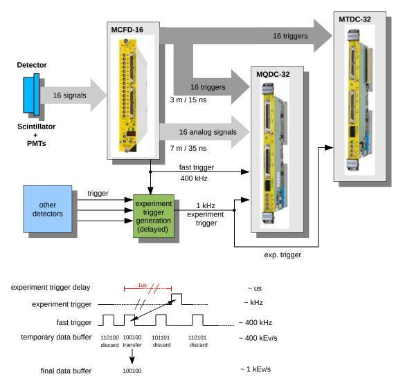
The 16 channel from PMT are connected vie 16 lemo cables to the inputs of an MCFD-16 discriminator.
