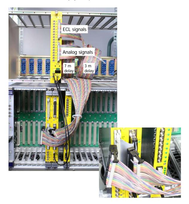
In the lower picture a crimp connector is added to the standard interface cable to connect to the MTDC input.
