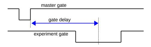
For the experiment gate the minimum low time (active) = 25ns, the minimum high time = 50ns.
