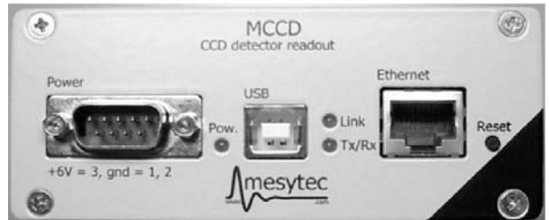
Front view of MCCD sequencer box: left the power input connector, middle the USB port and right side the Ethernet connector
