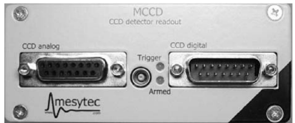
Rear side of the MCCD sequencer box: left and right connectors interface the CCD module. In the middle the Lemo 00 series connector can be used for external triggering of CCD sequence start or for output of internal trigger signal.
